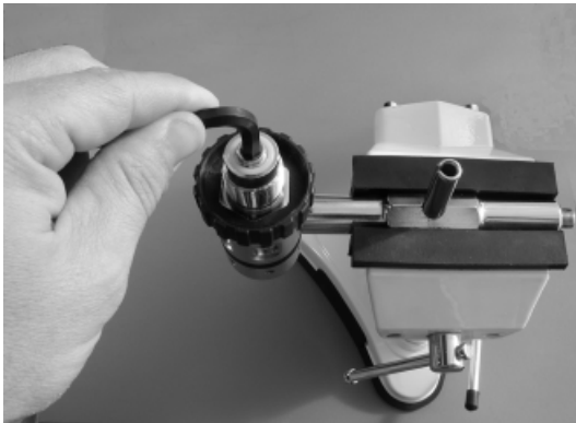
Fig. 5 – Removal of DIN Filter Retainer
