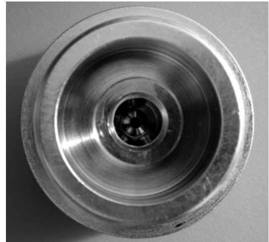
Fig. 7 – Inspection of Orifice Cone
