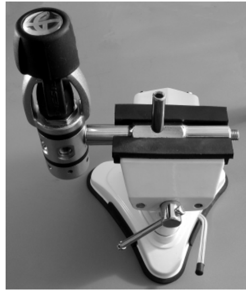
Fig. 1 – Recommended Vise Mounting
