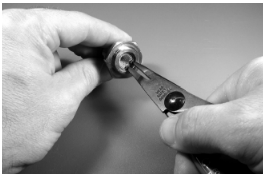
Fig. 4 – Removal of Filter Retaining Ring
