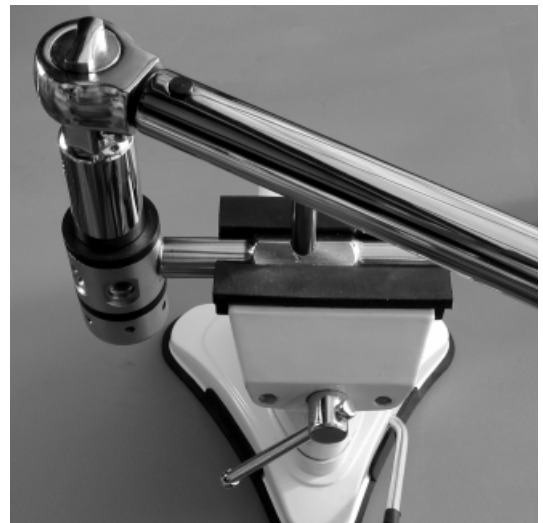
Fig. 11 – Torquing DIN Filter Housing
